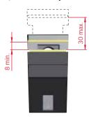
Shelf is clamped between a layer of ridged plastic on the lower side and soft rubber on the upper side (coloured parts).
